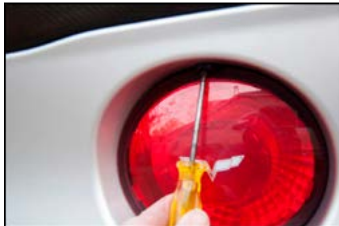
Fig 4a. Removing the Tail Lights
