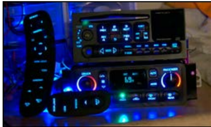
Fig 7c. Door switches, HVAC and radio
