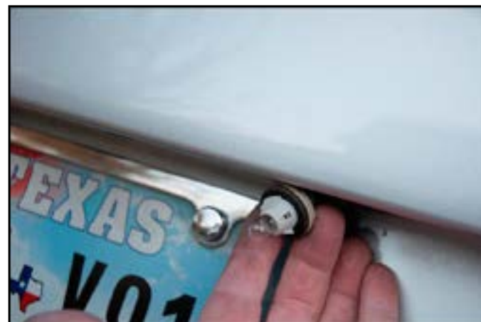
Fig 4b. The bulb harness
