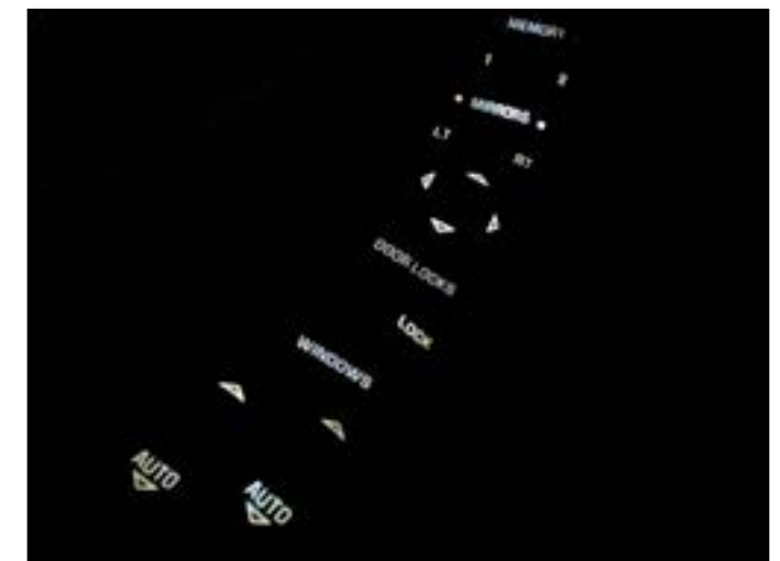
Fig 6a. Door switch LED
