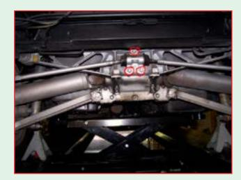
4. Now that the spring is out of the way remove the end links that attach to the center of the housing. I had to remove one end to remove the half shafts (that comes later) so I used a pickle fork and to swing it out of the way. Again important bolts are circled in red. The bolts are 15mm. Note: you will notice in a picture further down (2nd differential swap) that I left the rear spring attached when I dropped the batwing – your choice.
