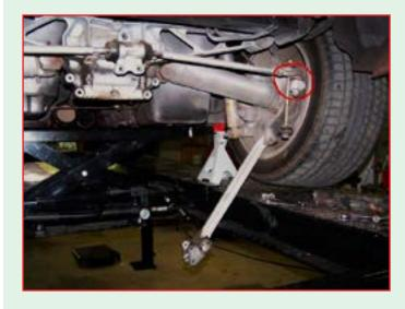
Next, remove the leaf spring. Do this by removing the side bolts first support the end of the spring with a jack and remove the nut and bushing. The bolt is 13/16 and the nut is 22mm. Take note of how many threads are showing as this is your ride height. You can take a floor jack to push up on the hub to release pressure on the bolt/nut.
