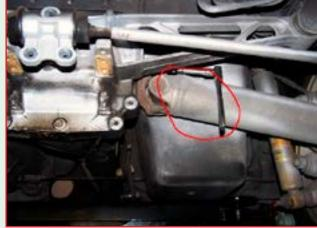
removing of the end link. Note: if you aren't replacing the u-joints, tape them with electrical tape to keep them from coming apart where you could lose your needle bearings. Note: this is where I decided to go ahead and replace the half shaft u-joints as well; and why not, one side is already disconnected.
